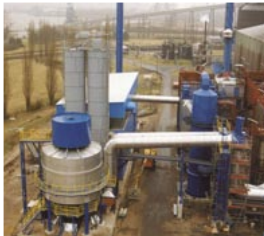
Dry sorption of HF with aluminium oxide and regenerative thermal post combustion
